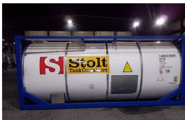
Figure 8.1: Views of ISO-Containers Used by BASF to Transport Acid Chlorides and Chloroformates
